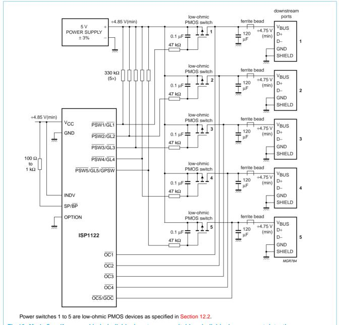
Fig 10. Mode 5: self-powered hub; individual port power switching; individual overcurrent detection.
